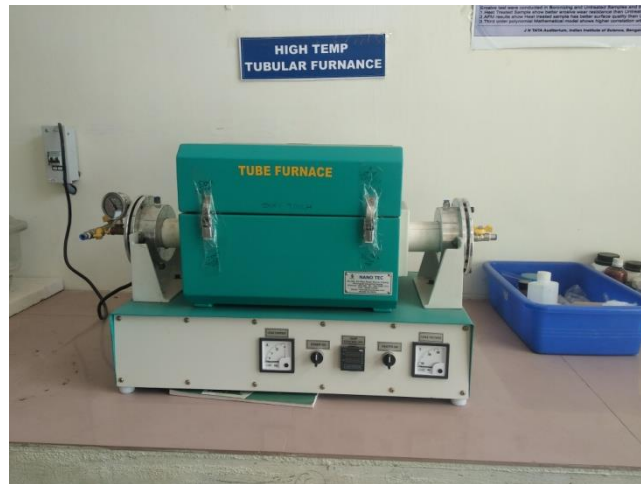
High Temperature Tubular furnace (Temp: up to 1200°C, Tolerance: \pm 1^\circ\text{C} )
